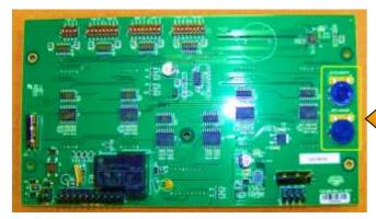
These two pots on the rear of the display board adjust the brightness of the red and blue score displays. Adjust the settings to suit your preferences.
